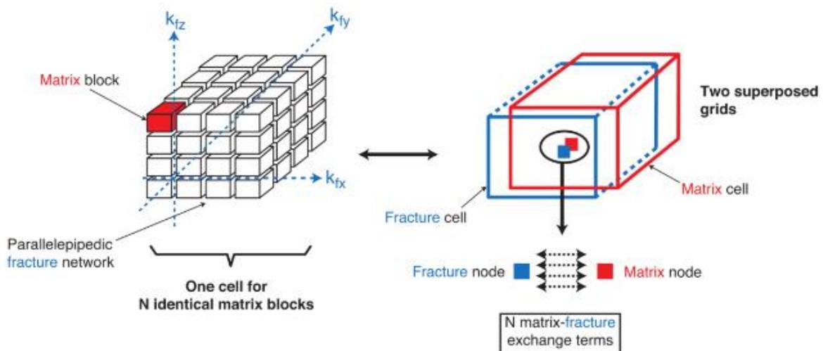
*Dual-porosity concept to represent a fractured reservoir in field-scale numerical simulations (from [3])*
