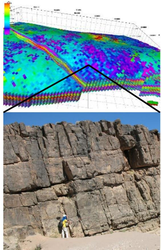
*Reservoir model and an outcrop example of a fractured carbonate formation. The properties of this fractured need to be averaged so that they can be represented by a single grid block in a reservoir simulation*
